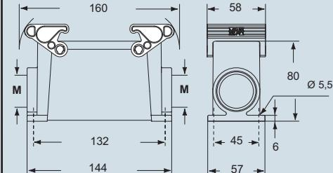
The surface mounting, high construction housings are supplied with an open threaded entry and diametrically opposite a closed threaded entry which can be opened by the user if required (with suitable tool).
