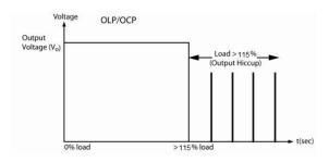
Additionally, if the  $l_0$  is < 115% but > 100% for a prolong period of time (depending on the load), the Over Temperature Protection (OTP) will be activated due to high temperature on critical components. The power supply will then go into "Hiccup mode" until power supply cool down.
