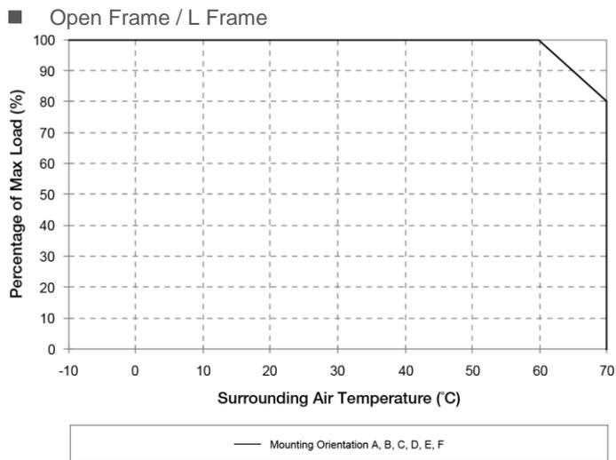
Fig.1.3 De-rating for Mounting Orientation A to F
