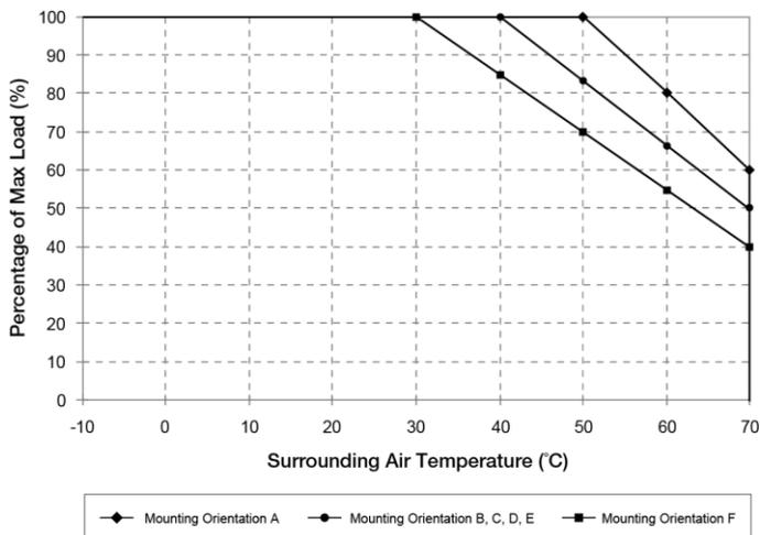
Fig.1.1 De-rating for Mounting Orientation A
