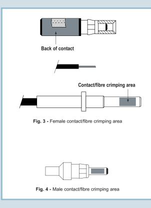
Insert the contact together with the fibre optic cable as far as possible into the crimping opening of the crimping tool (CLPZ R, see Figure 5) while applying gentle pressure to the fibre optic cable and connector, close the tool until you hear it disengages.
