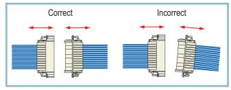
To keep the play within this limit, especially during the uncoupling phase, guide pins CRM and CRF may be used. The use of ILME pliers (code number CPES) is recommended for the uncoupling operations for CD inserts (64 poles) and CDD inserts (108 poles). The pliers work on the fulcrum and lever principle and perform the following main tasks:
