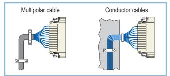
If the conductor bundles or the multipolar cables have to be immediately folded over on the back of the connector insert, it is recommended not to use any mechanical force in the axial direction with respect to the coupled contacts. The figure herebelow shows a correct bending and clamping of the multiwire bundles using the crimp contacts.
