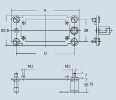
1) distance for electric and fibre optic contacts: max 27 mm distance for pneumatic contacts: max 26,5 mm
