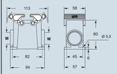
The surface mounting, high construction housings are supplied with an open threaded entry and diametrically opposite a closed threaded entry which can be opened by the user if required (with suitable tool).
