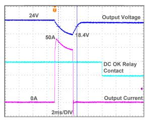
Fig. 8.2 APB 500% of nominal output current for 2ms
