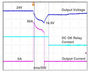
Fig. 8.3 APB 500% of nominal output current for 5ms
