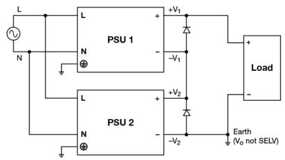
Fig. 11 Series Operation Connection Diagram
