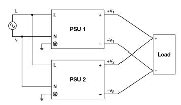
Fig. 10 Parallel Operation Connection Diagram
