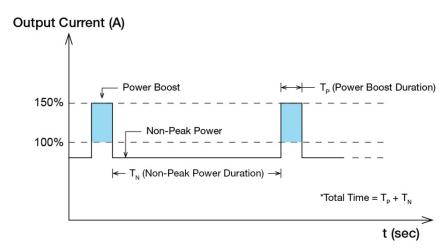
Fig. 7 Duty Cycle Calculation
