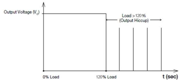
Additionally, if the  $I_o$  is  $< 120\%$  but  $> 100\%$  for a prolonged period of time (depending on the load), the Over Temperature Protection (OTP) will be activated due to high temperature on critical components. The power supply will then go into "Hiccup mode" until power supply cool down.
