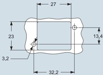
panel cut-out for CQS IA - CQS IAP enclosure, in mm
