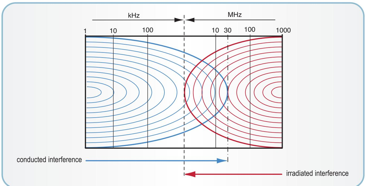
By test convention, **interference with frequency up to 30 MHz** is considered to be conducted and **irradiated with frequency above 30 MHz up to 1 GHz**.
