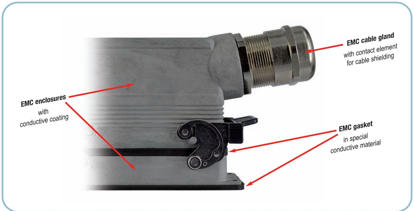
The enclosure surfaces are treated to make them extremely conductive while maintaining the necessary corrosion resistance. The bulkhead mounting housing has a special conductive gasket. For best results the surface underneath the gasket should be conductive.
