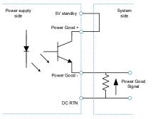
Figure 18. Power good signal connection
