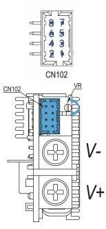
Figure 10. -x1 Module Connector
