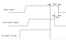
Figure 19. Power good signal sequence
