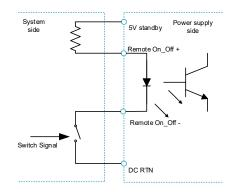
Figure 17. Remote On\_Off connection
