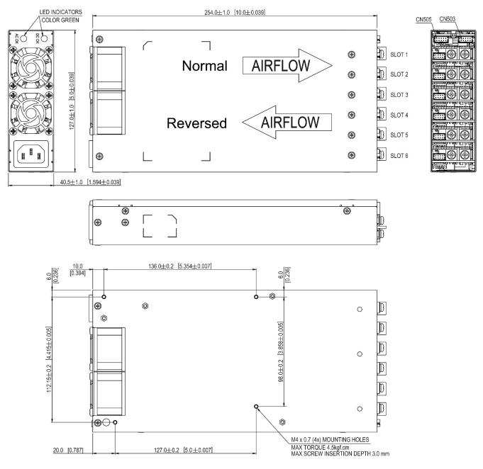
Figure 2. Dimensional drawing MEG-2K1A
