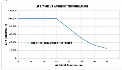
Note: Test at input voltage 220Vac, full Load.
