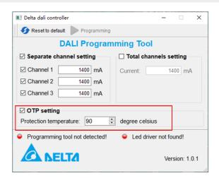
The trigger point of the lamp over temperature protection can be set easily. According to the actual conditions of the lamp, the user can set it between 90  $^{\circ}$ C and 120 $^{\circ}$ C through the computer control interface and communication tools. More details refer to User Manual.
