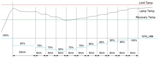
Note: This protection is an optional function, user can connect nothing to NTC connector in the junction box to ignore it. This protection requires the application of a special temperature detection circuit to realize the over-temperature of the lamp. The circuit is as follows.
