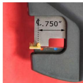
Wire Crimped in Hand Termination Tool
