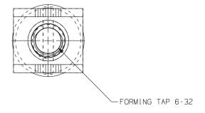
Typical PCB Mounting Detail [6.60] .130 .060 [3.30] [1.52] .120 [3.05] .160[4.06]Ø
